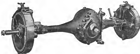
Fig. 2.—Front view of rear axle showing gear carrier, spring bases, and brakes, comprising the complete unit.
